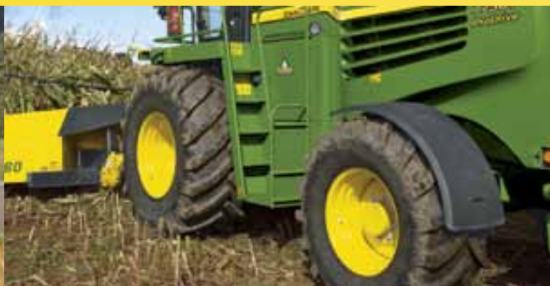
Independent axle speeds prevent sensitive soils from damage during headland turns
