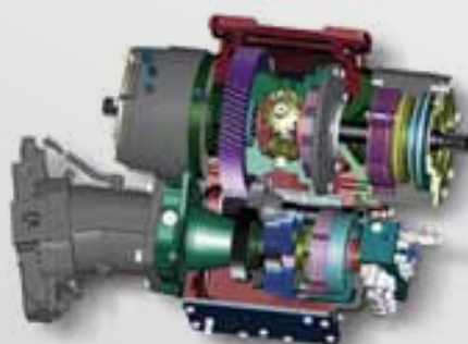
John Deere's ProDrive transmission is fully automatic which can automatically adjust driving speed in the field or on the road to match working conditions without increasing engine speed.
