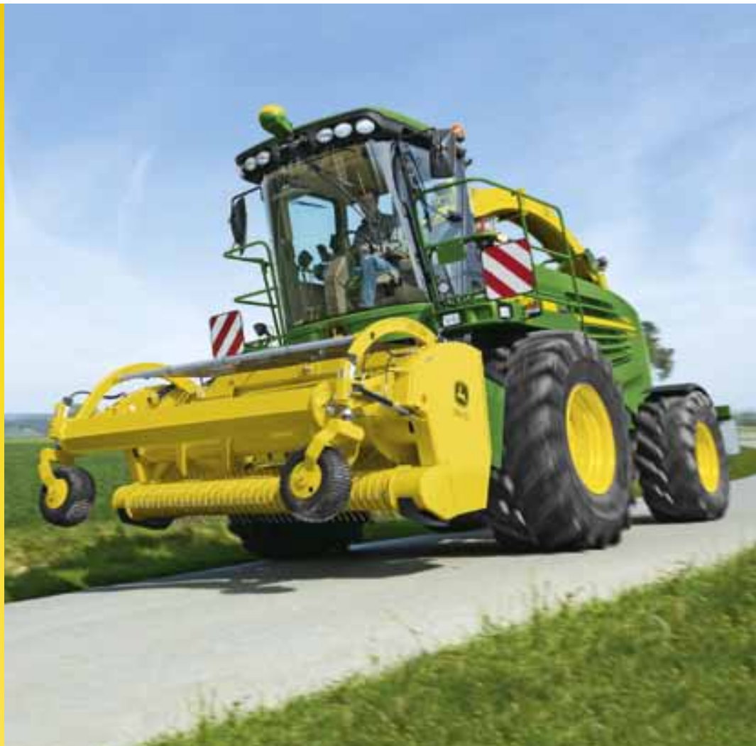
John Deere's ProDrive transmission is fully automatic which can automatically adjust driving speed in the field or on the road to match working conditions without increasing engine speed.
