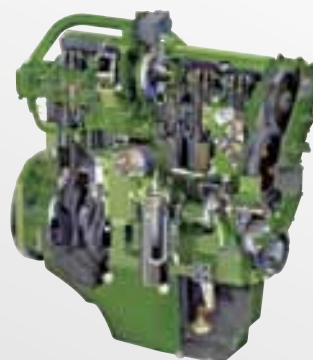
The 7080 Series forage harvester's John Deere PowerTech Plus™ engine which meets Stage III B emissions regulations, feature a variable geometry turbocharger that reduces consumption and boosts torque at low engine speeds. As a result, the forage harvester is less sensitive to sudden changes in field conditions or crop density.
