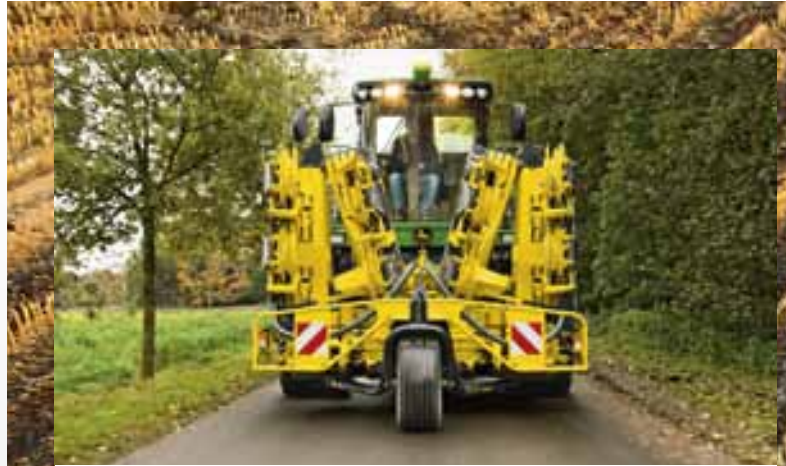
Folding to within 3.3 m width limit, even the 390plus is easy to transport with its centre support wheel.
